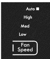
Note: Fan speed starts at high and adjusts to a slower speed as the room temperature dictates. For example, if the room doesn't get too warm it will stay at the slowest speed. If the room temperature rises quickly, such as when a door is opened, it will automatically go to the highest speed. The fan speed will re-adjust back to the slowest speed as the room returns to the original set temperature.
